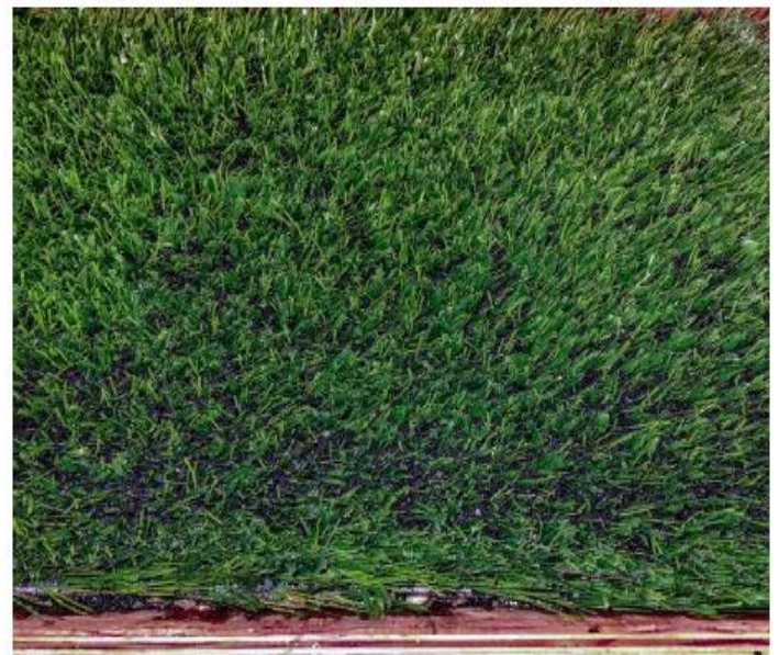
CAN003472 – System B (Generic SBR + Sand) overview (top) and close-up (bottom)
