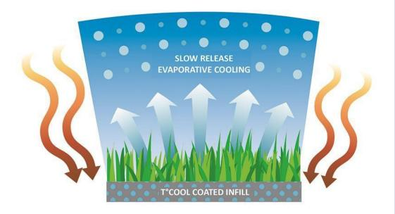
As the temperature rises, T°Cool<sup>TM</sup> releases moisture to create a cooling effect
