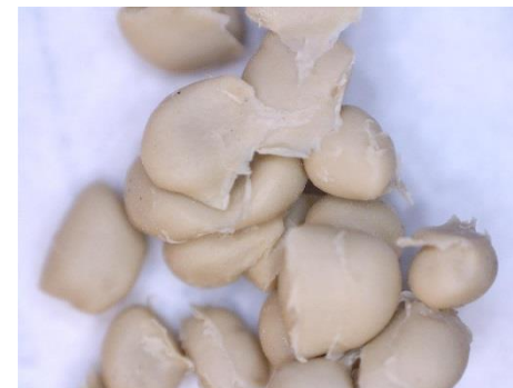
Material heated to 135 °C then cooled down
